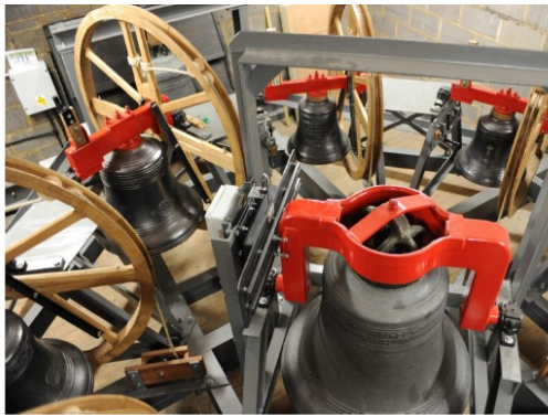
NEW PEAL OF EIGHT IN RADIAL FRAME TOGETHER WITH ELECTRICALLY SWUNG BOURDON AND STATIONARY SERVICE BELL, SOUTH OCKENDON.
